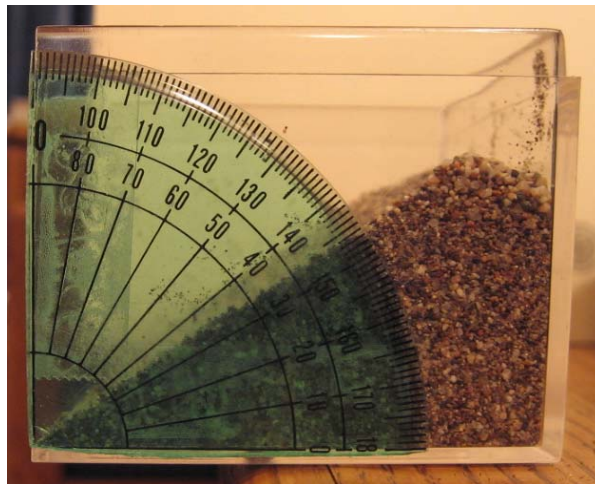
Figure 7. Drained-angle-of-repose test of sand from one of the larger dunes.
