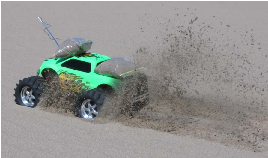
Figure 13. Climbing a 7^\circ slope carrying sand-bags representing a 50% increase in mass (shortly before getting stuck).
