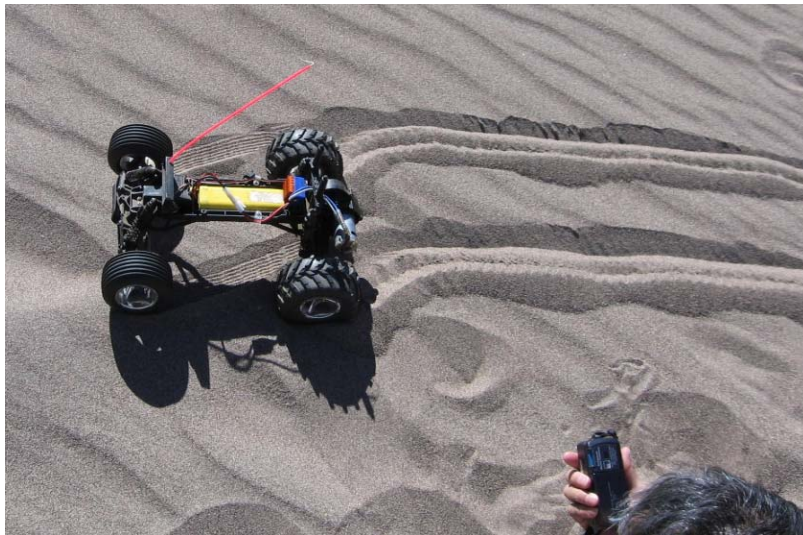
Figure 11. Rover #84, slipping diagonally across a dune face as an angled climb up an approximately 14^\circ dune face is attempted.
