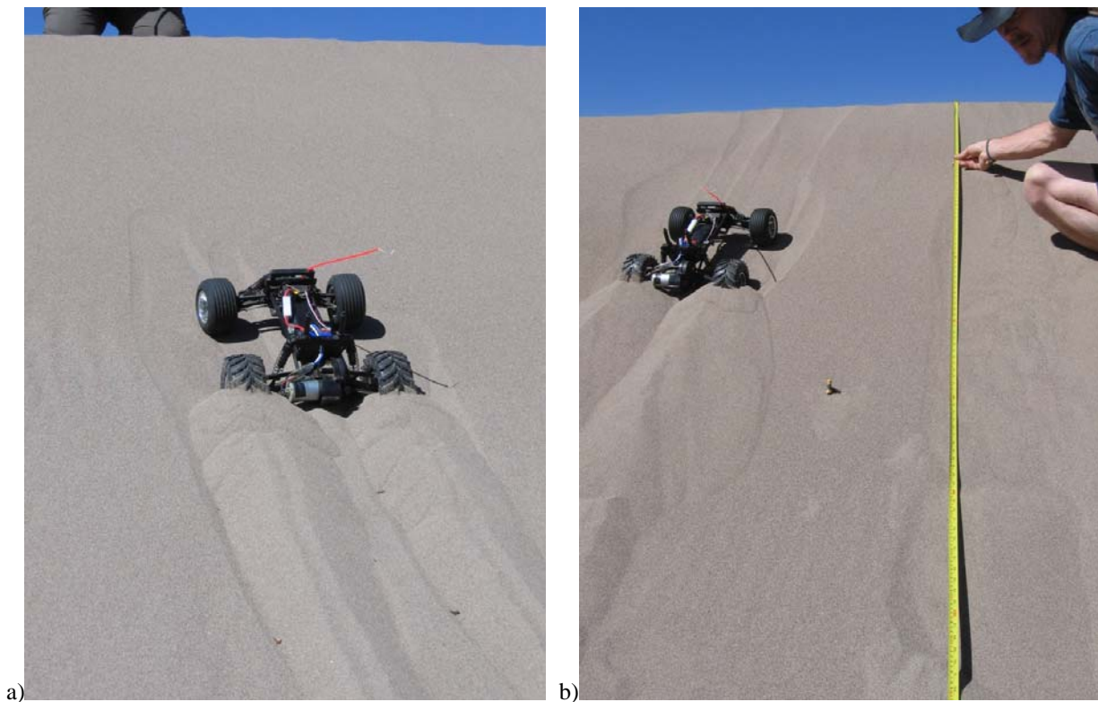
Figure 14. Rover #84 climbing up the steep face of a dune at \sim 4\text{mm/s} by building an 'avalanche-ladder' (piles of sand behind each slowly spinning rear tire, fed by small avalanches flowing in from well in front of the rear tires). (a) top of the left avalanche is well in front of the left-front tire, while right avalanche lags behind. (b) both avalanches extend to the crest of the dune.
