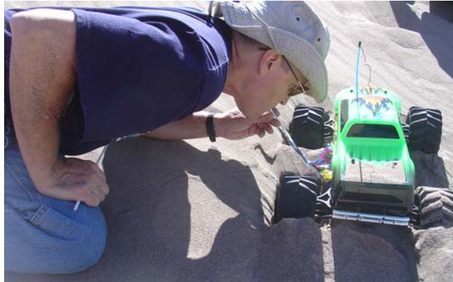
Figure 10. Using a mylar balloon to jack up the ‘Green Machine’ after it was stuck,
