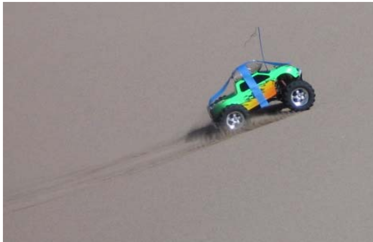
Figure 12. The Green-Machine Rover carrying a 25% load up a 19^\circ slope at high speed
