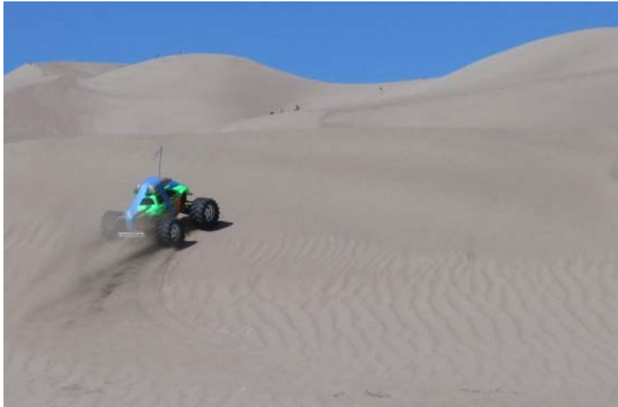
Figure 1. A fast rover, dubbed the Green Machine, speeding toward the crest of a dune loaded with a sandbag weighing 25% of the weight of the unloaded rover, including its batteries.
